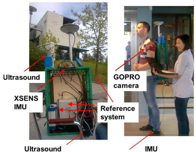
Figure 2: Test setup and equipment
