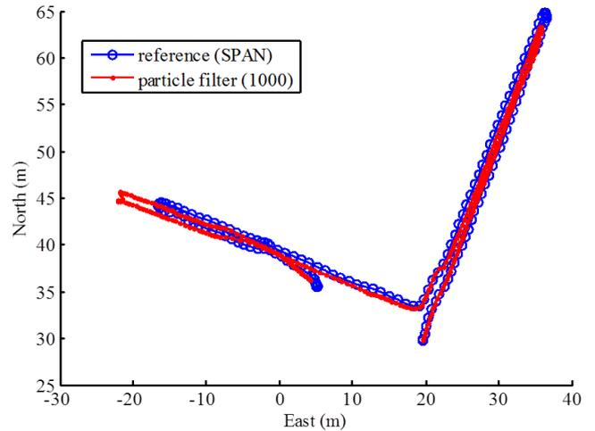
Figure 5: Particle filter fusion results compared with the SPAN reference trajectory in horizontal plane.
