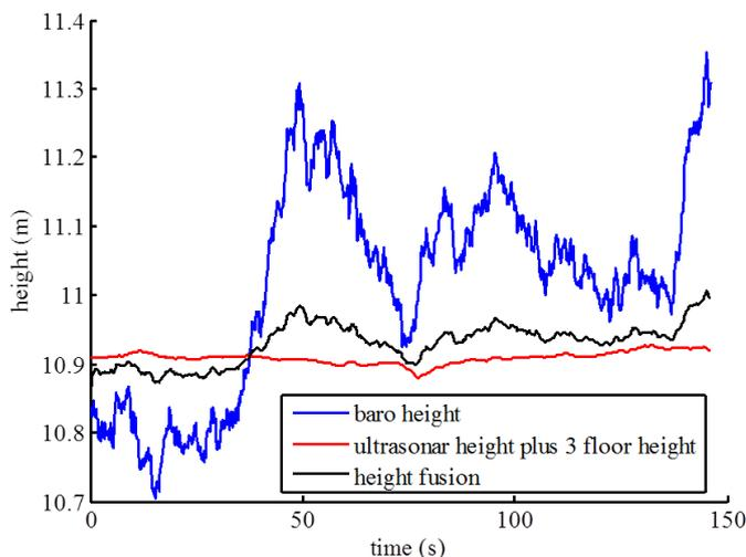
Figure 6: Barometer and sonar height and the fusion results
