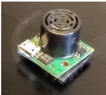
Figure 4: Ultrasonic ranging sensor HRUSB-MaxSonar used in the experiments
