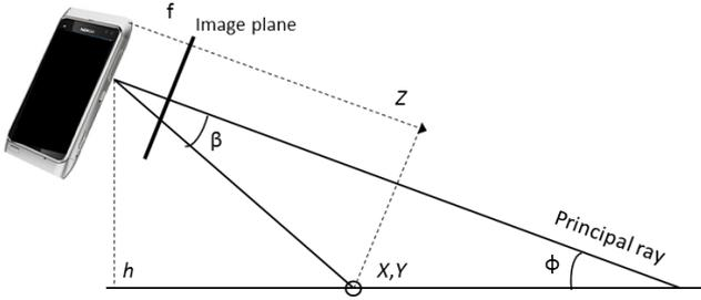
Figure 1. Special configuration of the camera for resolving the depth of the objects in images.
