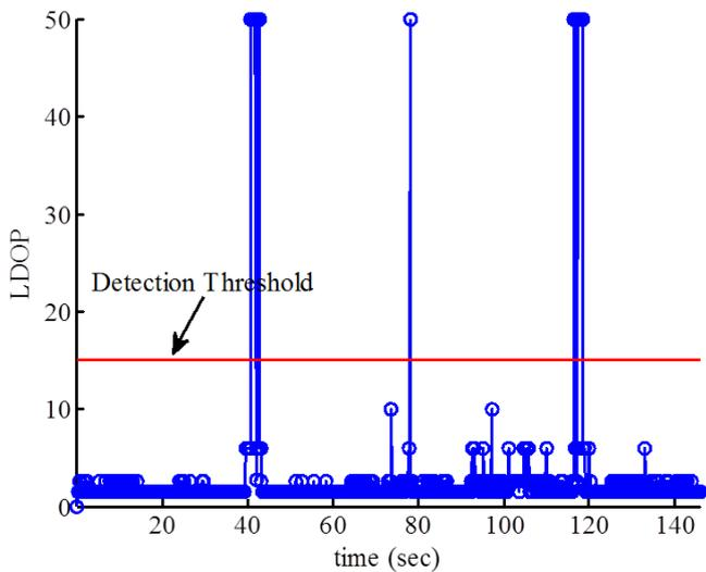
Figure 3: Visual gyroscope’s LDOP values in the experiment and the threshold for rejecting the visual measurements
