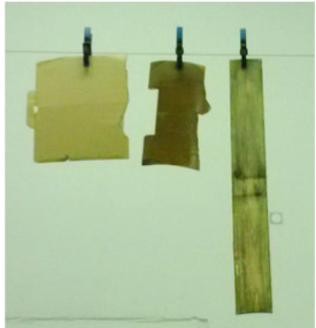
Fig. 3. The targets hanging on a wire in the scanned area. The wet and dry cardboard samples are in the left and middle, respectively.
