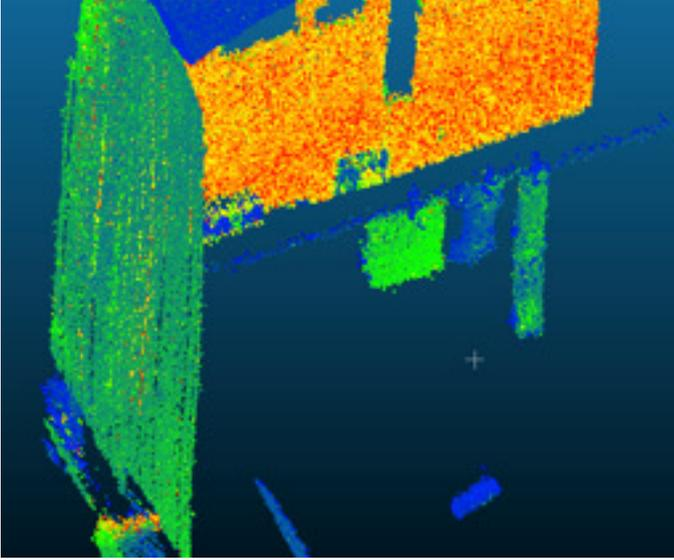
Fig. 4. The HLS point cloud (plotted with CloudCompare Version: 2.6.1) of the laboratory corner with the targets visible in the middle of the image. The point cloud is shown with intensity in one of the Near-Infrared channels.
