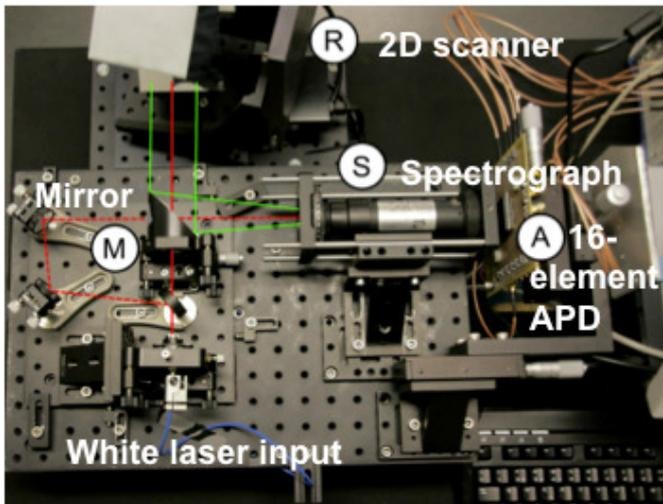
Fig. 1. The FGI hyperspectral lidar (HSL) optical setup: Red beam: White laser input. R: 2D scanner. M: Off-axis parabolic mirror. S: Spectrograph. A: 16 element avalanche photo diode array.
