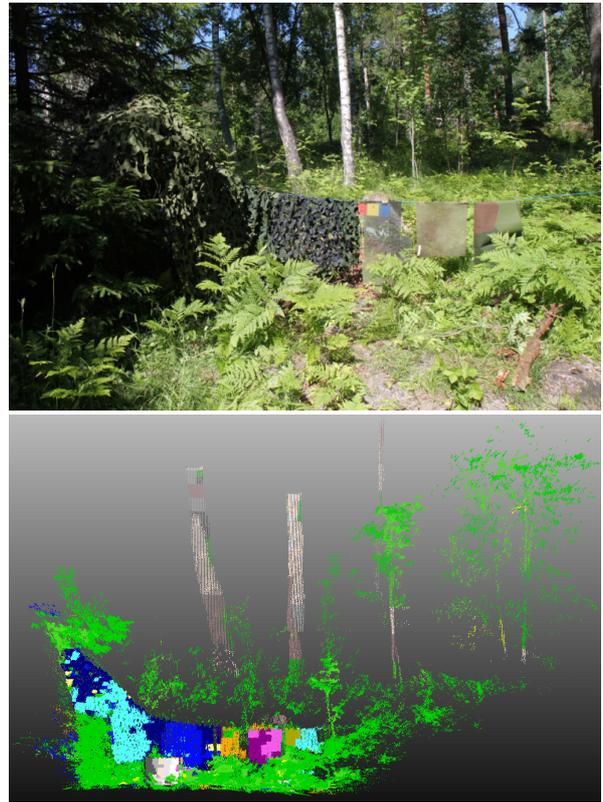
Fig. 2. Target identification with the FGI hyperspectral lidar (HSL), showing the capability of the instrument of detecting targets in the scanned area using spectral libraries.
